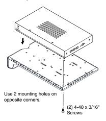
2. Secure the device to the plate with 4-40 screws.
